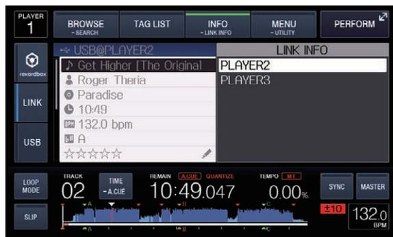
When another DJ player is connected by PRO DJ LINK, the details of the track loaded on the other DJ player can be checked.
