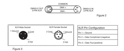
Special Note: Line Termination. When longer runs of cable are used, you may need to use a terminator on the last unit to avoid erratic behavior. A terminator is a 110-120 ohm 1/4 watt resistor which is connected between pins 2 and 3 of a male XLR connector (DATA + and DATA -). This unit is inserted in the female XLR connector of the last unit in your daisy chain to terminate the line. Using a cable terminator (ADJ part number Z-DMX/T) will decrease the possibilities of erratic behavior.
