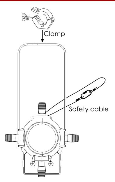
The Performer can be placed on a flat stage floor or mounted to any kind of truss with a clamp.
