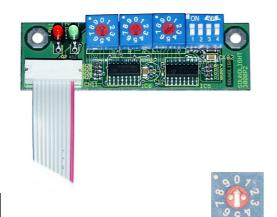
A DMX start address board is required to set the DMX start address and the DMX personality. A start address boars is NOT included with DIN rail mountable devices and must be ordered separately. The start address board can be used with all types of SOUNDLIGHT interfaces. At your option, a start address board 3000P (switches) or a start address board 3003P (LED display) can be used.
