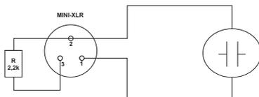
Headset, lavalier or wind instrument microphone with low output. 2,2 kOhm resistor soldered on pin 2 and pin 3 increases gain.
