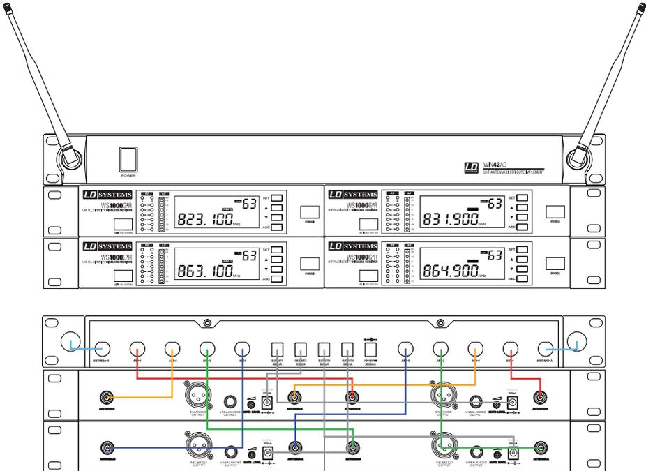
The antenna divider LDWIN42AD (optional) can handle up to 4 LDWS1000G2R single receivers or up to 4 LDWS-1000G2R double receivers.
