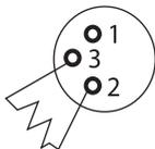
Use of a terminating resistor (termination) reduces interference and other problems during signal transmission. It is always advisable to connect a DMX termination module (resistance 120 ohms, 1/4 W) between pole 2 (DMX-) and pole 3 (DMX+) of the last device in the chain.
